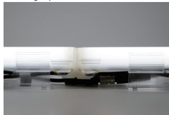
Connectors can be put under LED fixture
